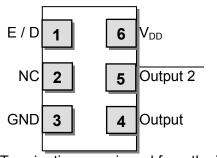
Terminations as viewed from the Top NOTE: XPRESSO LVDS XOs are designed to fit on Industry Standard, 6 pad layouts
